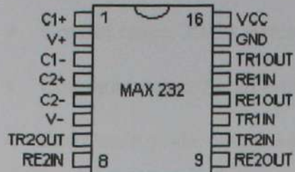
Figure 2.14: Pin outs for the MAX-232, RS-232 Driver/Receiver
