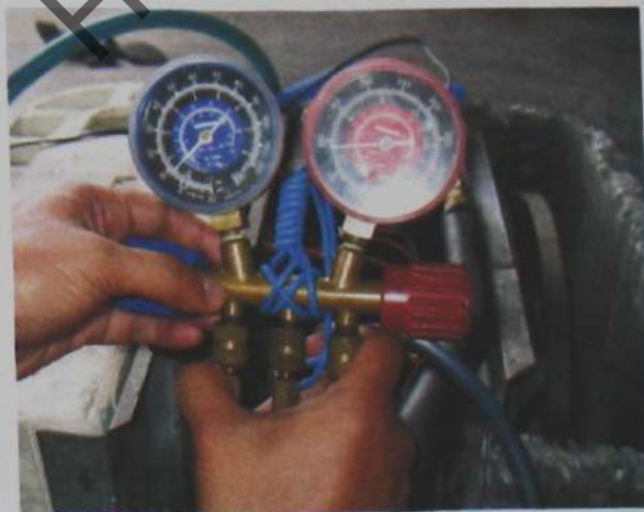
Rajah 3.18 : Ujian Prestasi Model ( Discharge Pressure, Suction Pressure, Condenser Inlet & Outlet Pressure, Evaporator Inlet & Outlet Pressure ) Sedang Dijalankan
