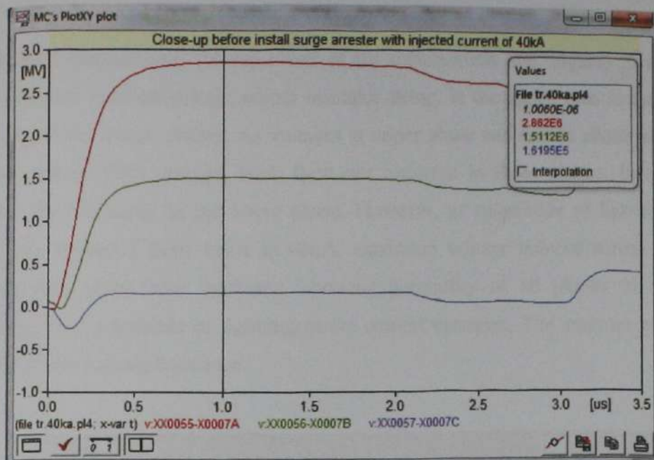
Figure 5.14: Close-up before install surge arrester with injected current of 40kA.
