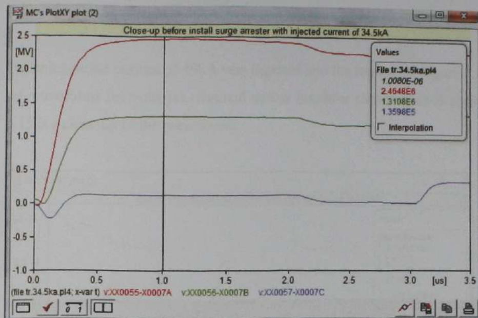
Figure 5.12: Close-up before install surge arrester with injected current of 34.5kA.
